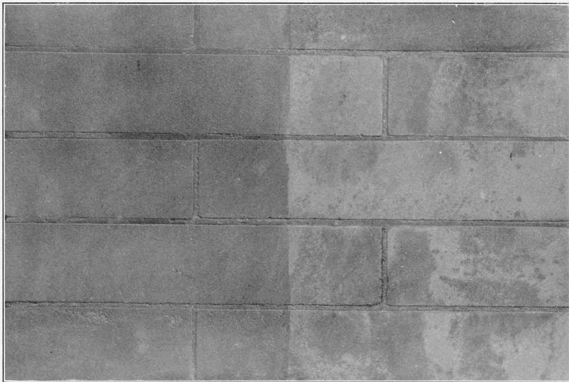
FIGURE 11.— Leaching test on limestone panel 1. Right-hand half treated with a 10-percent paraffin solution.
