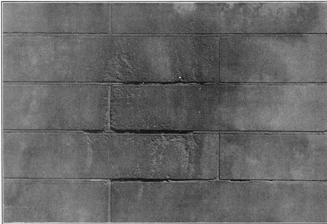
FIGURE 12.— Leaching test on limestone panel 3. Right-hand half treated with a 4-percent solution of aluminum soap.
