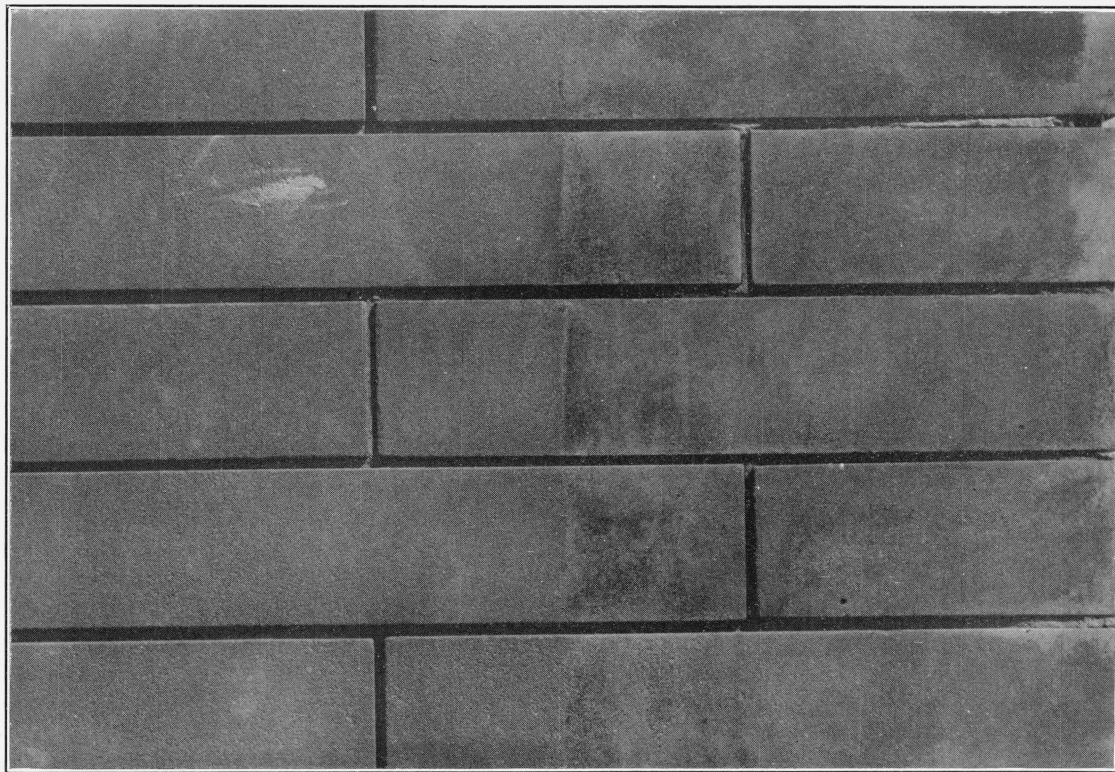
FIGURE 14.— Leaching test on limestone panel 7. Right-hand half treated with a 15-percent paraffin solution.
