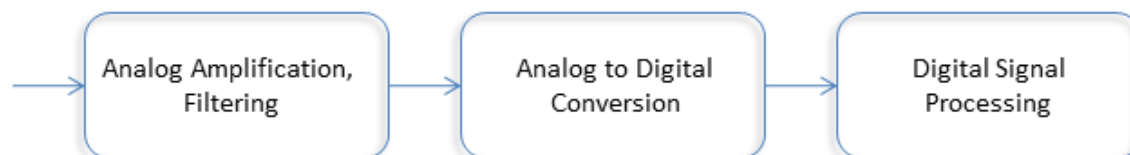
Fig. 1. Conventional mixed-signal analog-to-digital sampling architecture.
