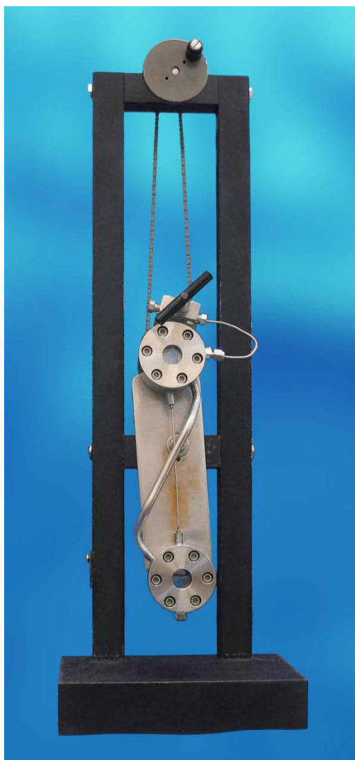
Fig. 4. Viscometer mounted on stand with crank.
