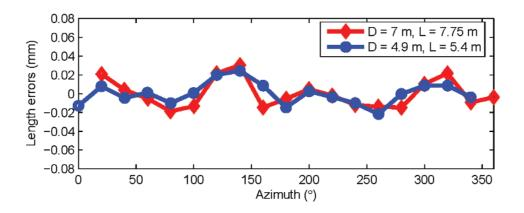
Fig. 7. Length errors (residuals from the mean length) are shown in the figure for horizontal length tests for two different combinations (D = 7 m, L = 7.75 m and D = 4.9 m, L = 5.4 m) after correcting the tracker map for second order errors in the scale. Data was collected from tracker A.
