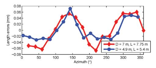
**Fig. 9.** Length errors (residuals from the mean length) are shown in the figure for horizontal length tests for two different combinations (D = 7 m, L = 7.75 m and D = 4.9 m, L = 5.4 m) with the original encoder map of the tracker (i.e., before correcting the tracker map for second order errors). Data was collected from tracker C.
