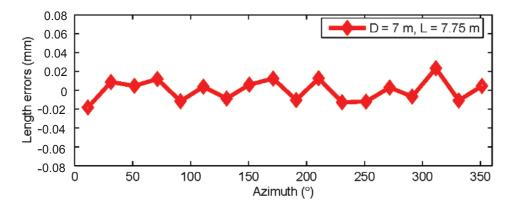
Fig. 12. Length errors (residuals from the mean length) are shown in the figure for horizontal length tests for tracker F. No second order scale error is noticeable.
