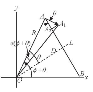
Fig. 2. Calculating the error in the length AB due to scale error in the encoder.
