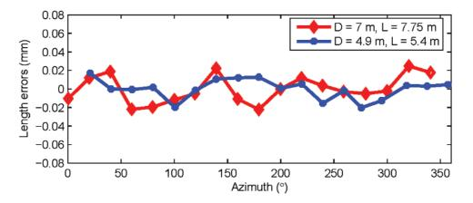
**Fig. 10.** Length errors (residuals from the mean length) are shown in the figure for horizontal length tests for two different combinations (D = 7 m, L = 7.75 m and D = 4.9 m, L = 5.4 m) after correcting the tracker map for second order errors in the scale. Data was collected from tracker C.
