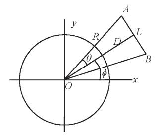
**Fig. 1.** Reference *AB* of length *L* positioned distance *D* from the tracker located at *O*. The range to the targets at *A* and *B* is *R*. The reference length *L* subtends an angle  $2\theta$  at the origin *O* and the bisector of *L* is located at an angle  $\phi$  from the *x* axis.
