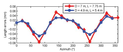
**Fig. 6.** Length errors (residuals from the mean length) are shown in the figure for horizontal length tests for two different combinations (D = 7 m, L = 7.75 m and D = 4.9 m, L = 5.4 m) with azimuths taken from the original encoder map of the tracker (i.e., before correcting the tracker map for second order errors). Data was collected from tracker A.
