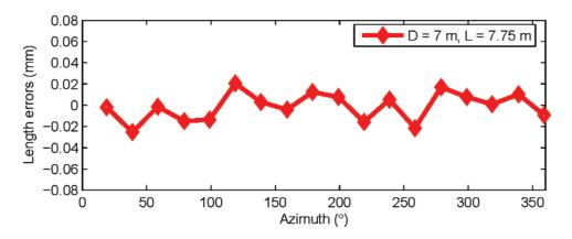
Fig. 11. Length errors (residuals from the mean length) are shown in the figure for horizontal length tests on a new tracker design (tracker E) that intrinsically compensates for second order scale errors. As expected, no second order scale error is noticeable.
