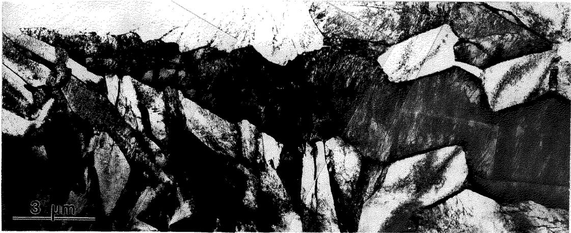
**Fig. 8.** Bright field TEM micrograph showing the detailed morphology of the needles shown in Fig. 8. The needles have very irregular interfaces. Blocky grains between elongated needles are most probably cross-sections of the needles with their long axes normal to the TEM foil.
