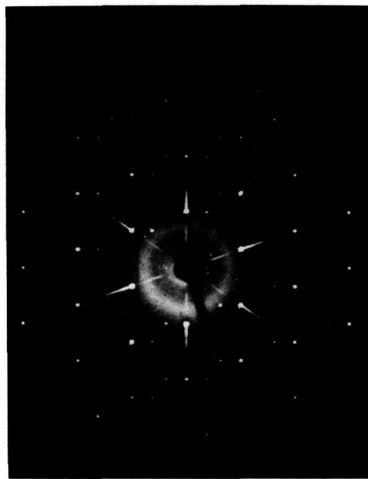
**Fig. 7.** X-ray precession photograph of the fcc  $\alpha_2''$  phase (Mo radiation).
