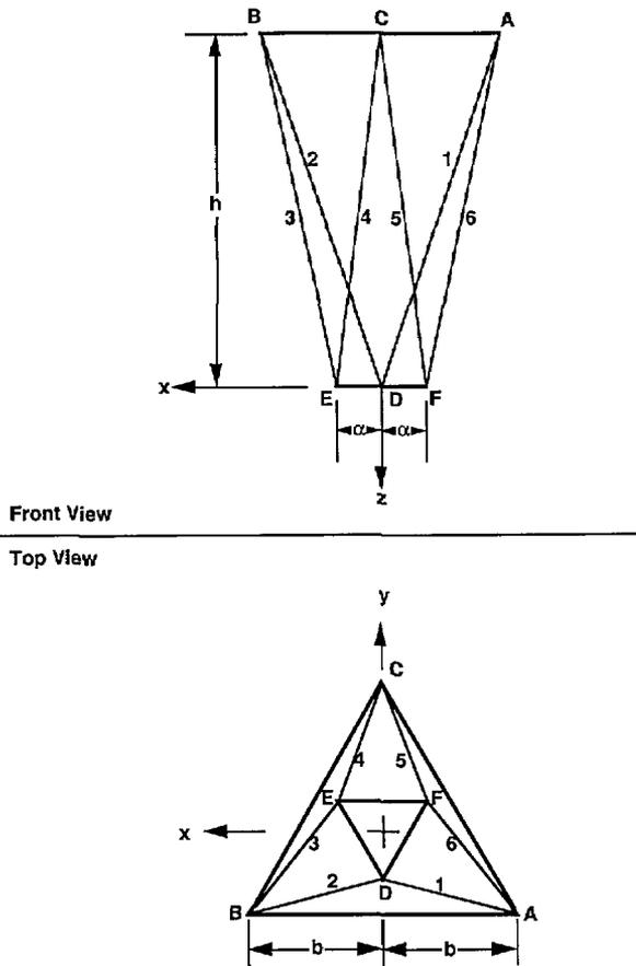
Fig. 8. Robot crane cable support structure.
