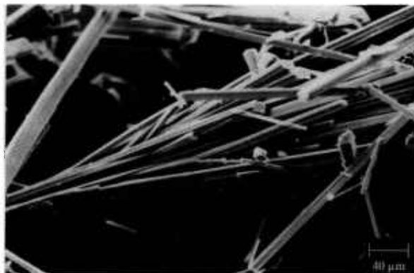
Fig. 1. Scanning electron micrograph of calcium hydrogenurate hexahydrate crystals.
