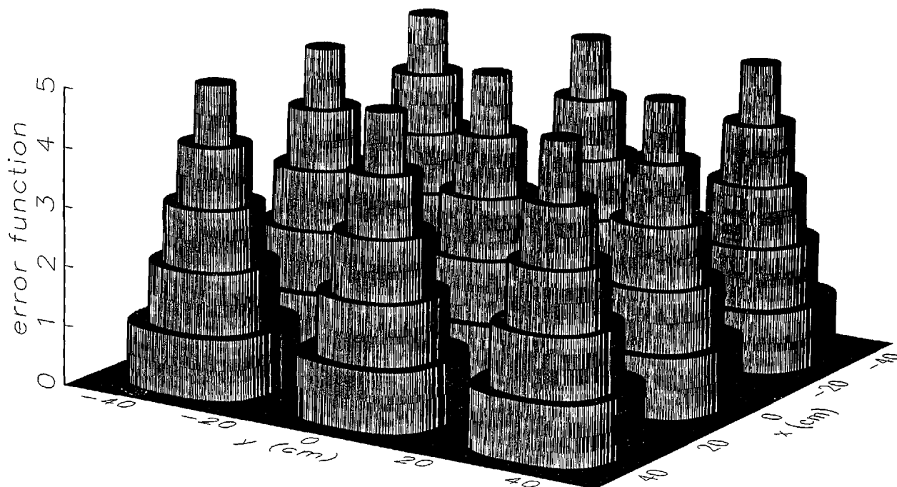
Fig. 7. The discrete probe position error function. The discrete error surface is given by z = \delta z \text{int}[N \cos^2(3\alpha x) \cos^2(3\alpha y) + 0.5] , where N=5 is the maximum scan plane index, int is the fortran truncate-to-integer function, and \alpha = 2\pi/L .
