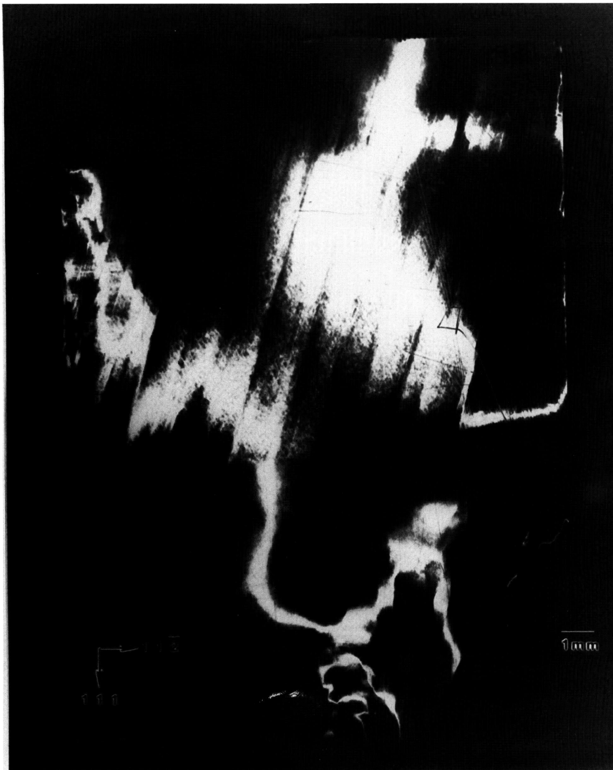
Figure 19. High-resolution (220) stationary diffraction image from the approximately (220) surface of terrestrial GaAs crystal in Bragg geometry. The growth direction is [111]. Lighter areas diffract more strongly.
