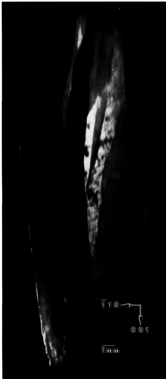
Figure 11. High-resolution (220) 8 keV diffraction image in Bragg geometry from the approximately (220) surface of PbSnTe crystal grown on STS 61A. The growth direction is [001]. Lighter areas diffract more strongly.
