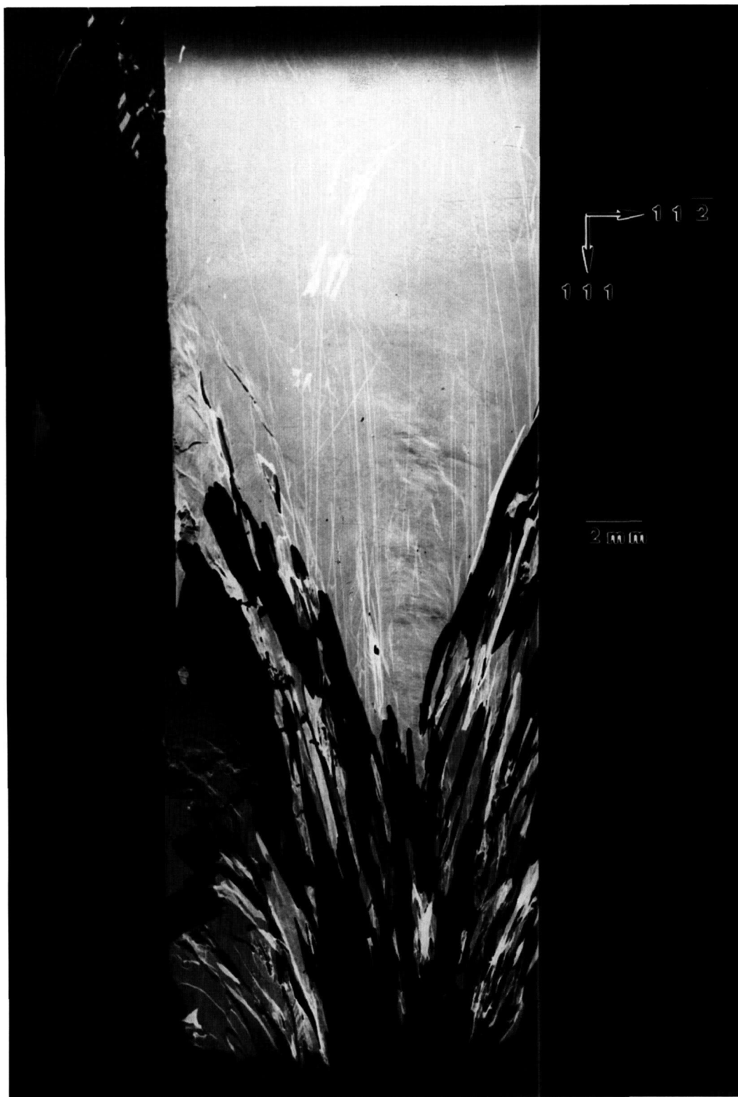
Figure 17. Low resolution (220) 8 keV diffraction image of the approximately (220) surface of terrestrial GaAs crystal, in Bragg geometry. The sample was rocked through an angle of 4^\circ during this exposure; the growth direction is [111]. Lighter areas diffract more strongly.
