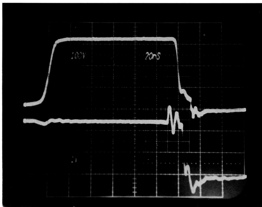
Figure 3. Voltage and current waveforms for sustained avalanche with second breakdown in MOSFET. Top trace: 100 V per small div.; bottom trace: 10 A per small div.; time: 20 ns per small div.
