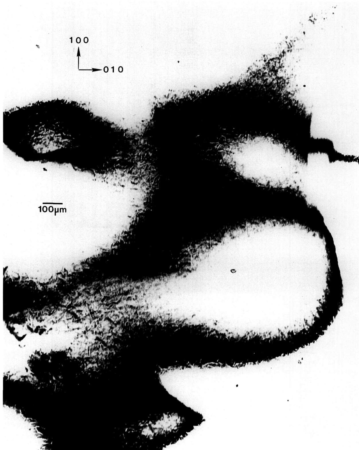
Figure 7. Enlargement of lower left portion on figure 6, (1 0 10) diffraction. Darker areas diffract more strongly.
