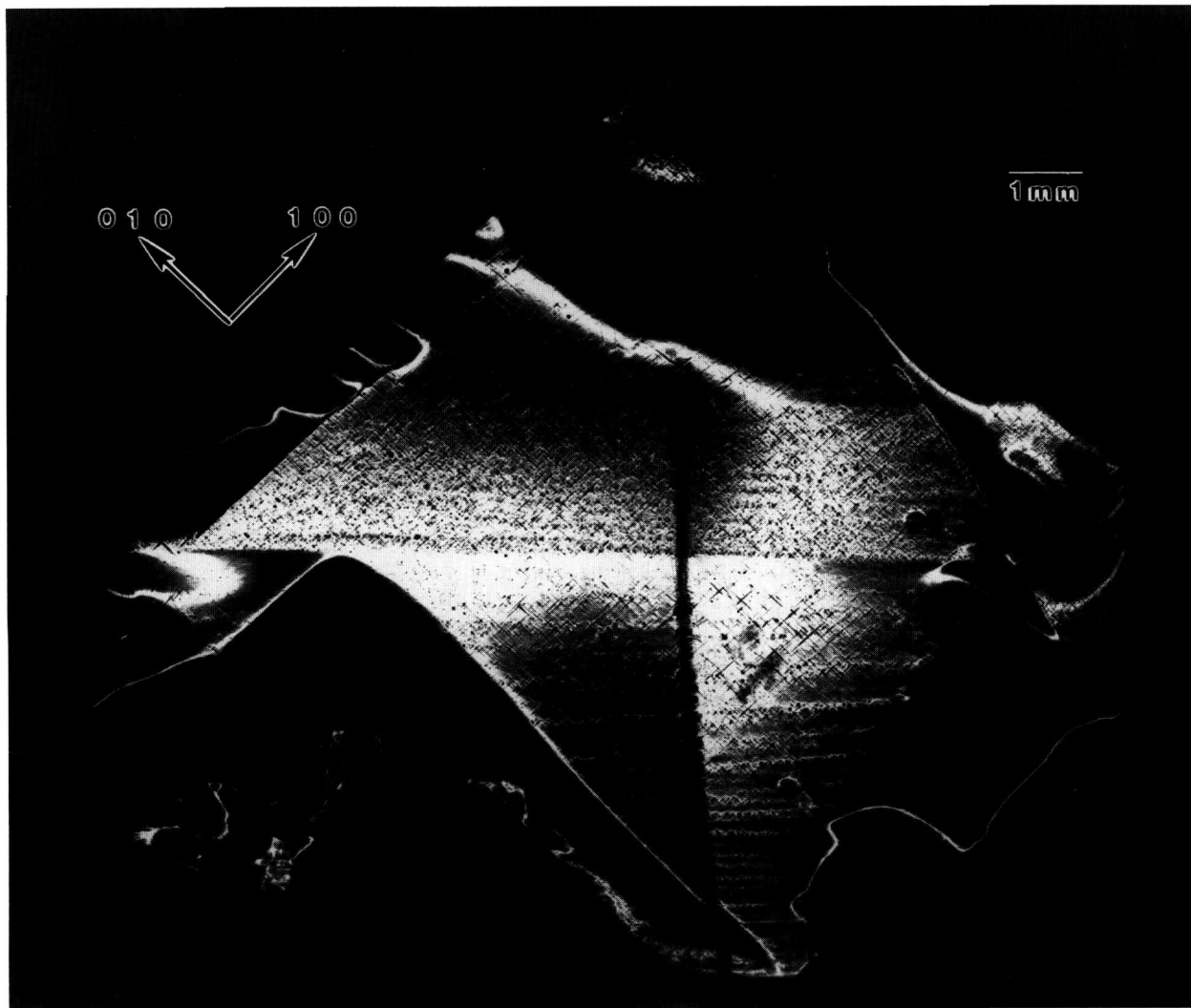
Figure 1. High-resolution (1 1 12) 8 keV diffraction image in Bragg geometry of the (001) surface of terrestrial \text{HgI}_2 crystal comparable to that grown on Spacelab III. Lighter areas diffract more strongly.
