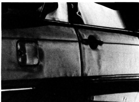
Figure 2. Comparison of a new car body viewed without D-sight (above) and with D-sight. The shadows in the images are caused by minute form deviations of the part. Taken from the work of Pryor et al. (paper 14).
