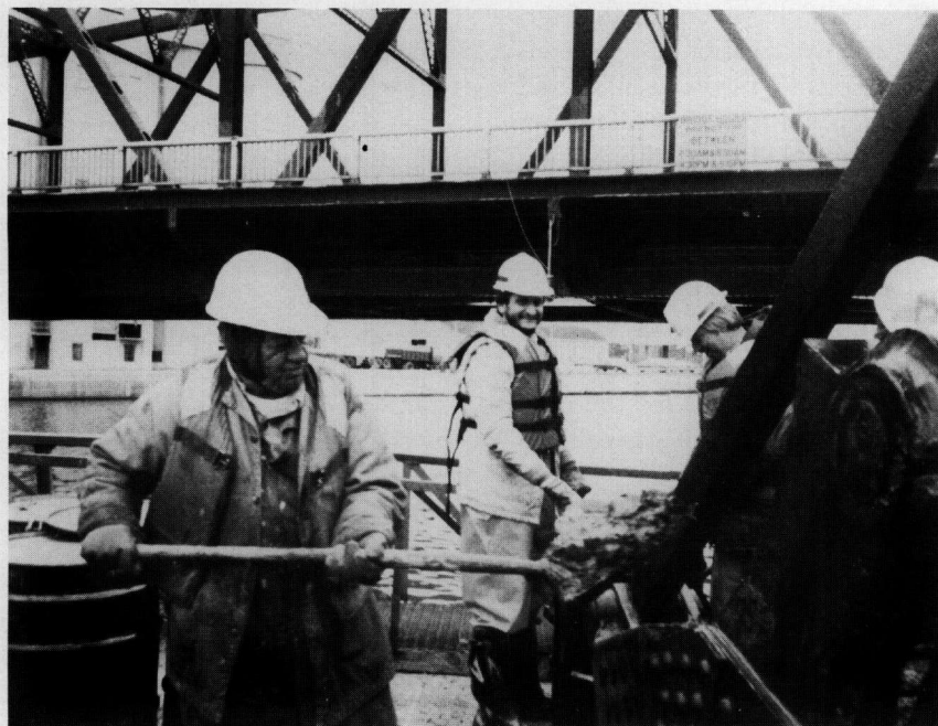
Figure 1. River sediment being transferred from collection bucket to teflon-lined barrels using teflon-coated shovels.
