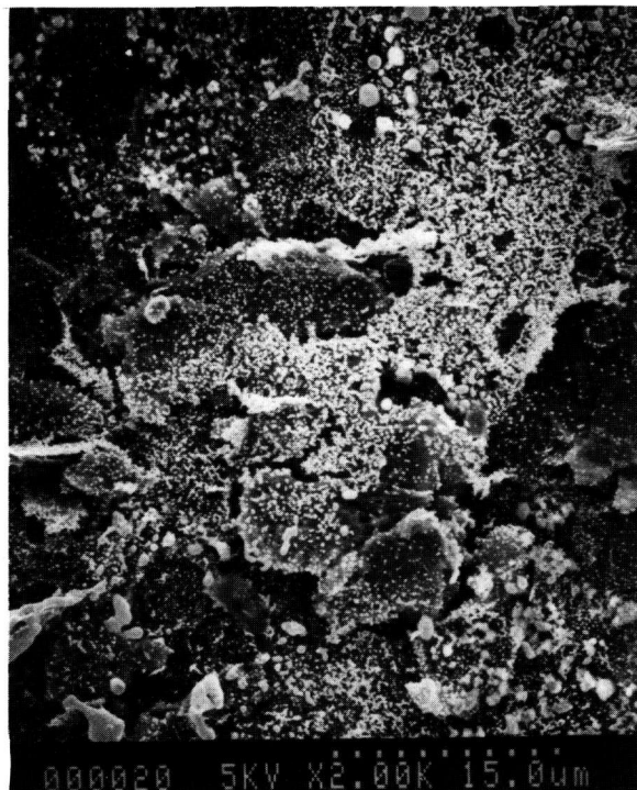
Figure 1. Scanning electron micrograph of reduced palladium metal on graphite surface (20,000x magnification).
