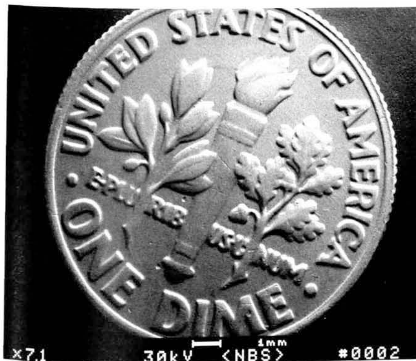
Figure 2 —Scanning electron micrograph of a dime demonstrating the importance of proper SEM calibration procedures. Note that the magnification is displayed in the lower left corner and the accelerating voltage displayed in the center. See text for full explanation.
