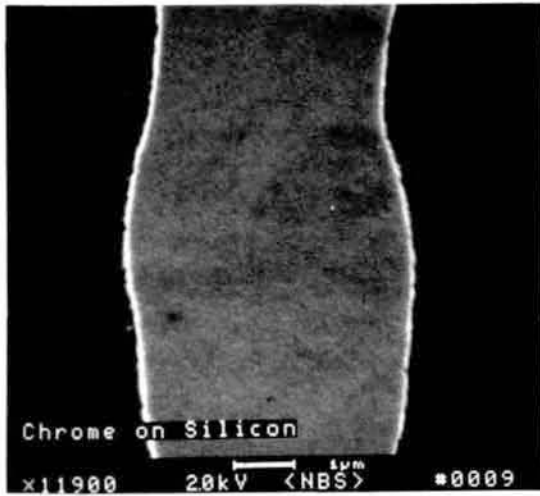
Figure 9 —The effects of non-synchronized ac field induction on the image in an SEM. (a) Micrograph taken under ambient conditions where the instrument is synchronized to line (60 Hertz). (b) Micrograph taken after induction of a non-synchronized field that is 1/4 cycle off of 60 Hertz. Note the broadening of the structure.
