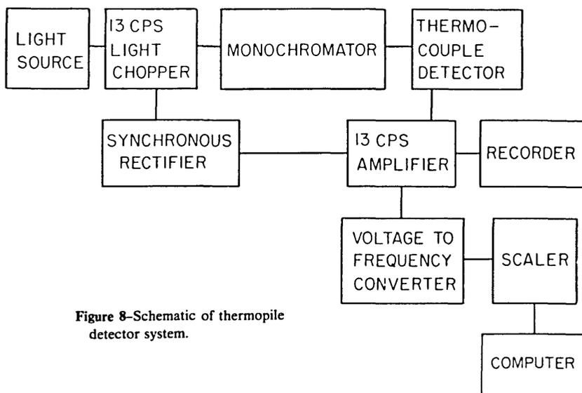
Figure 8—Schematic of thermopile detector system.
