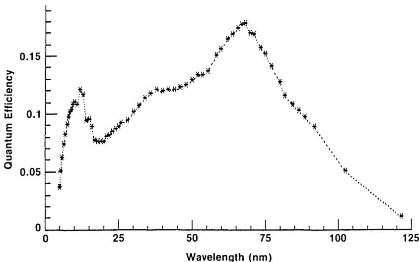
Figure 2—Typical quantum efficiency of NBS windowless photodiodes.
