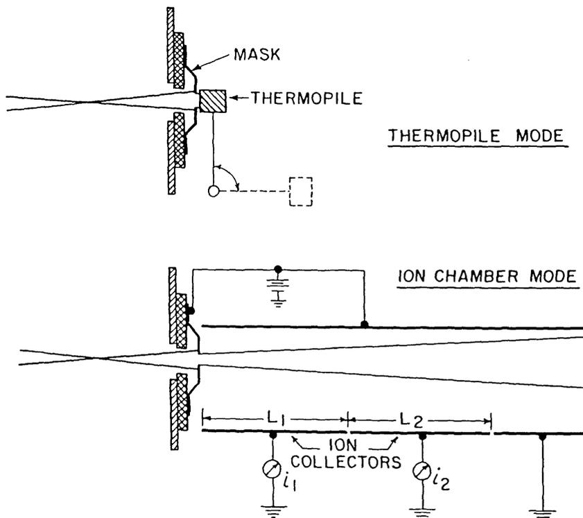
Figure 4—Configuration of thermopile and ionization chamber detectors.
