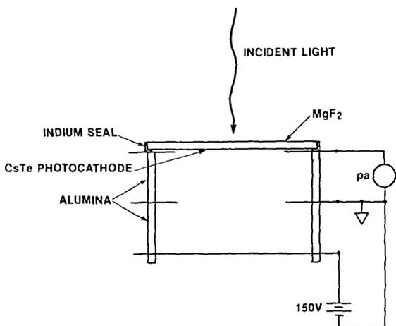
Figure 3—Schematic and wiring configuration of EVSD photodiode.
