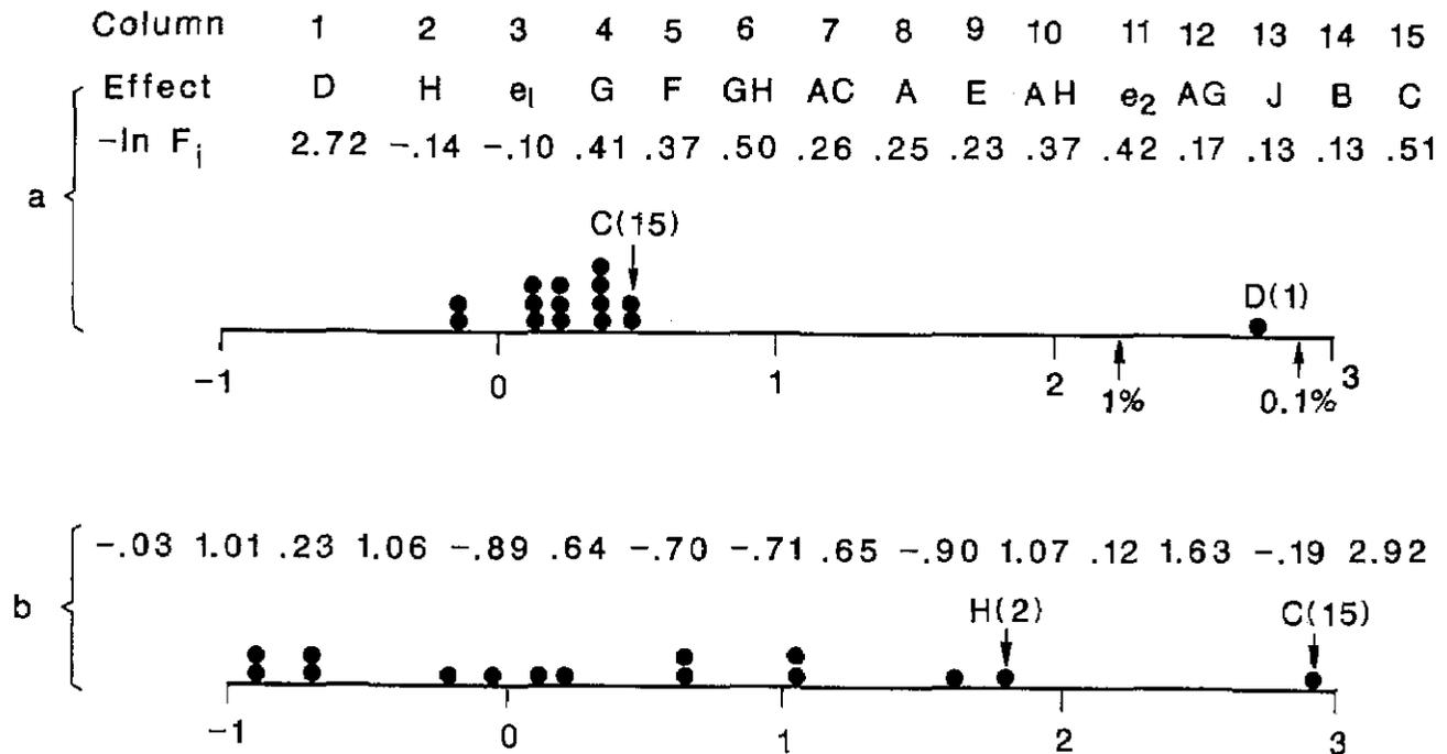
**Figure 2**—Welding experiment log dispersion effects (a) before, and (b) after elimination of location effects for B and C.
