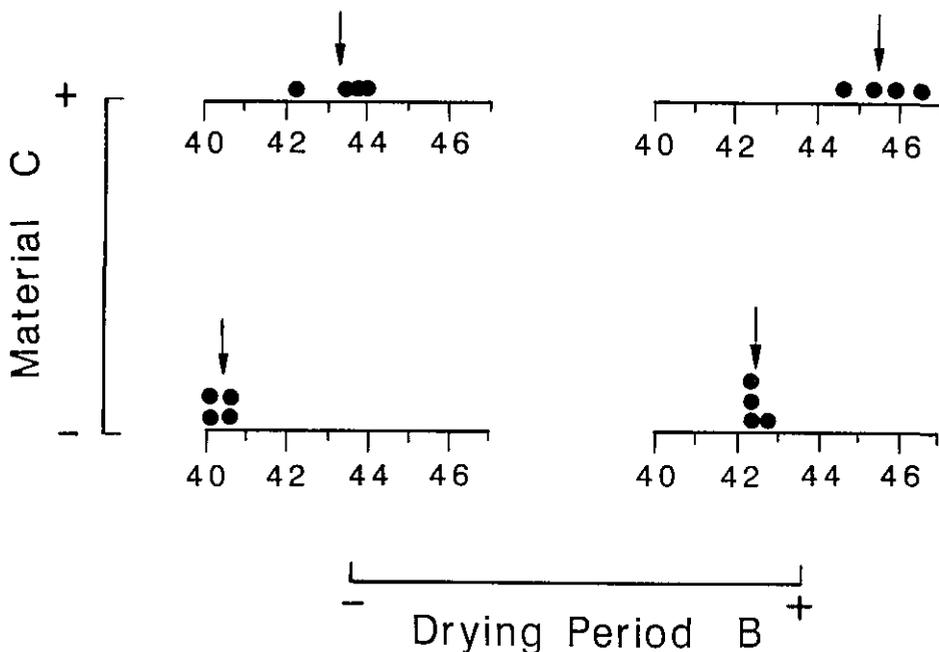
Figure 1—Tensile strength data as four replicates of a  $2^2$  factorial design in factors B and C only.
