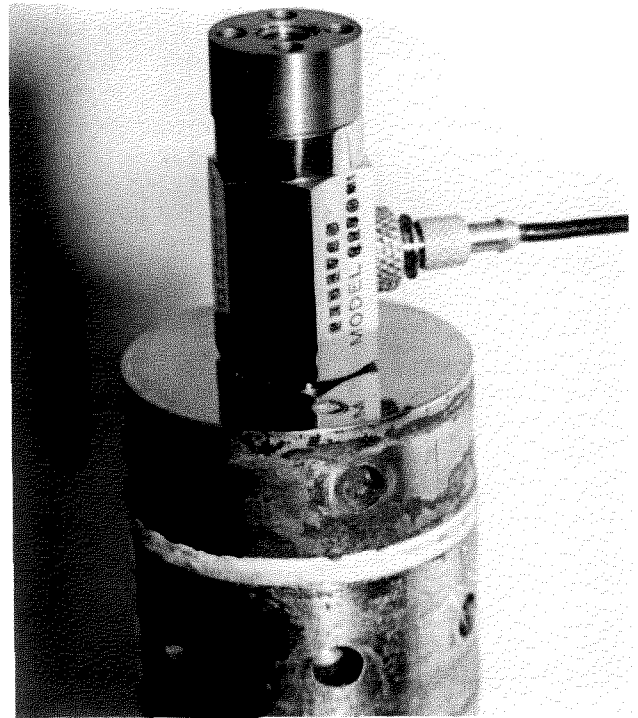
Figure 4-A back-to-back accelerometer with a dummy mass mounted for optical calibration.
