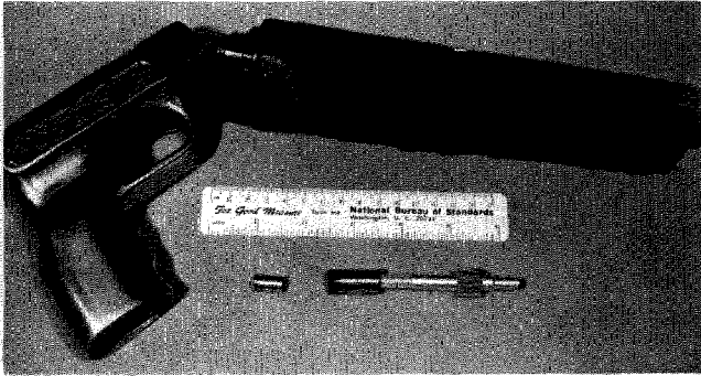
FIGURE 11. Windsor probe apparatus showing the gun, probe and blank cartridge.
