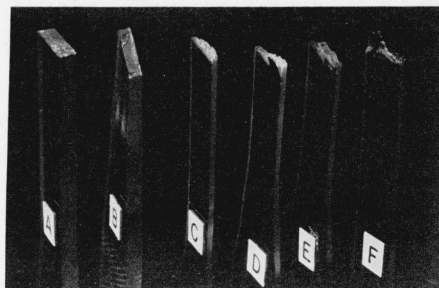
FIGURE 6. Effect of biaxial stretch-forming to about 50 percent elongation on the fracture of tensile specimens
