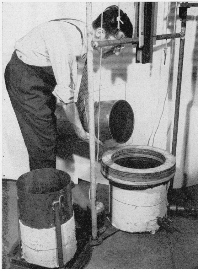
FIGURE 3. Vacuum-forming apparatus partly disassembled after forming a sheet of acrylic plastic. The formed piece is on the end of the form which is held by the operator.
