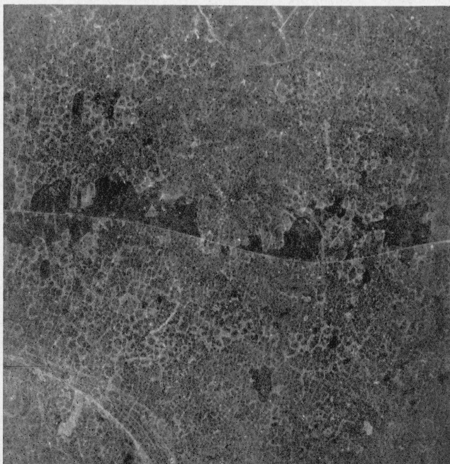
FIGURE 12. Mosaic structure formed on surface of mica crystals after heat treatment.
