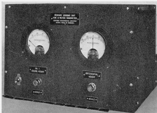
FIGURE 2. Mercury-sensing unit for 8-meter manometer.
