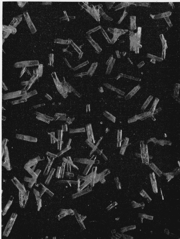
FIGURE 3. \text{BaO}\cdot\text{Al}_2\text{O}_3\cdot 4\text{H}_2\text{O} , prismatic form.
