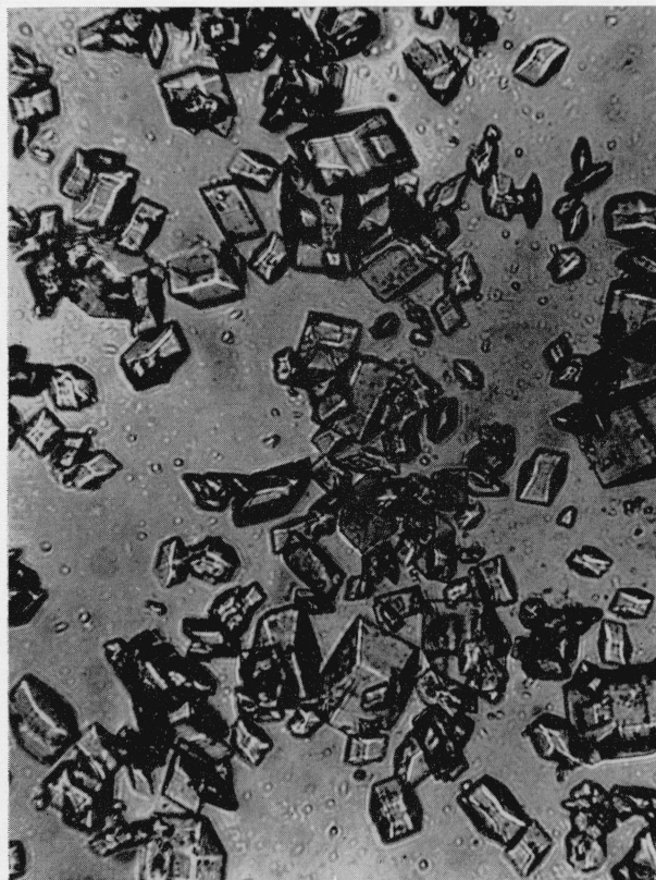
FIGURE 4. \text{BaO} \cdot \text{Al}_2\text{O}_3 \cdot 4\text{H}_2\text{O} , rhombohedral form. Magnification, \times 250 .
