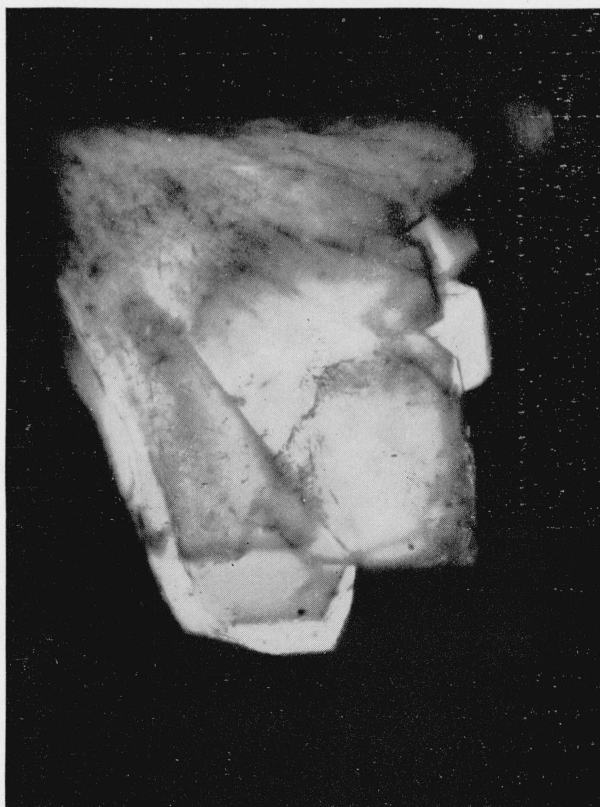
FIGURE 5. \text{BaO} \cdot \text{Al}_2\text{O}_3 \cdot 2\text{H}_2\text{O} . Crossed nicols, magnification, \times 100 .
