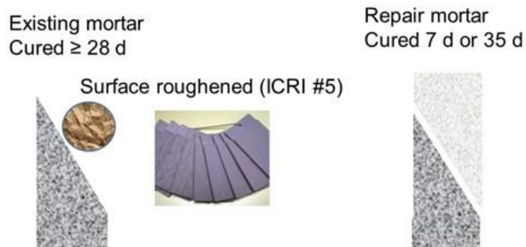
Figure 1. Schematic of preparation of specimen for shear slant testing.
