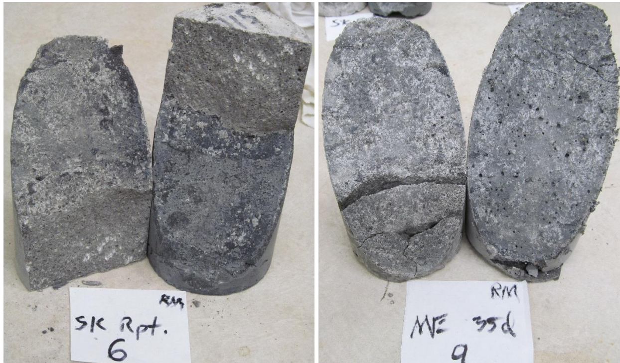
Figure 12. Photos of typical specimens after shear slant testing. Some strong bonding of the two materials is indicated by the deposits of one material on the opposing material face. The (darker) repair material half specimen is on the right in both images.
