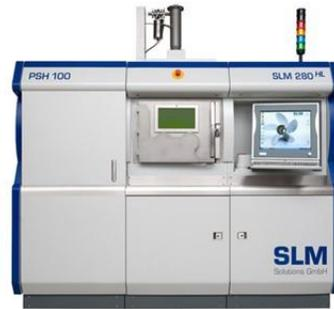
Selective Laser Melting (SLM) Machine, SLM Solutions
