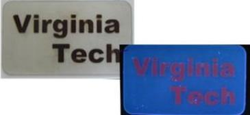
*Material Jetting of 0.5wt% Quantum Dots*
