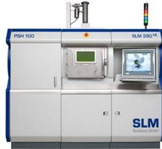
Selective Laser Melting (SLM) Machine, SLM Solutions
