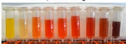
CdSe QDs in UV light (365 nm)
