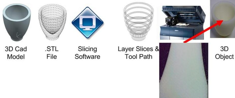
3D Cad Model    .STL File    Slicing Software    Layer Slices & Tool Path    3D Object
