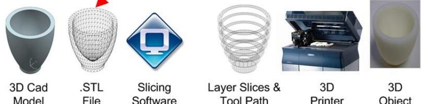
3D Cad Model    .STL File    Slicing Software    Layer Slices & Tool Path    3D Printer    3D Object
