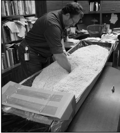
Figure 3-18. Spreading Bedding Material the.
