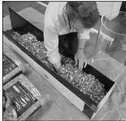
Figure 3-20. First Pour into the Test Measure.
