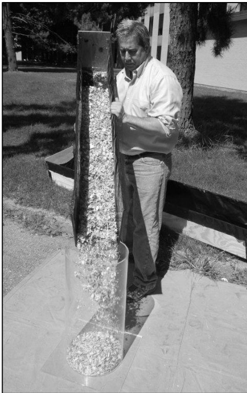
Figure 3-23. Filling a 44 L Test Measure.
