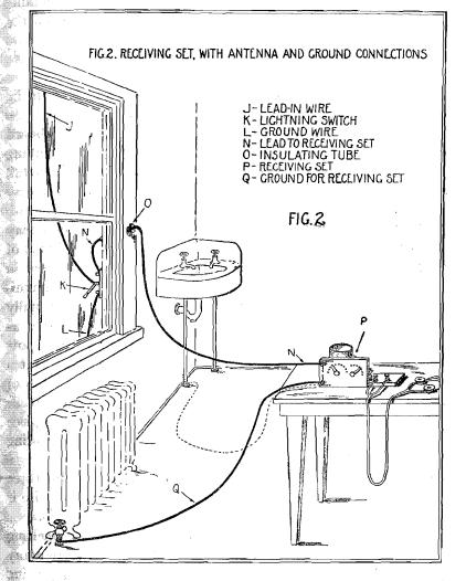
metallic conductor to the ground. If there are no water pipes or radiators in the room in which the receiving set is located, the wire should be run out of doors and connected to a special ground below the window. The ground for the lightning switch should not be used for this purpose. It is essential that for the best  $97966^{\circ}-22-2$
