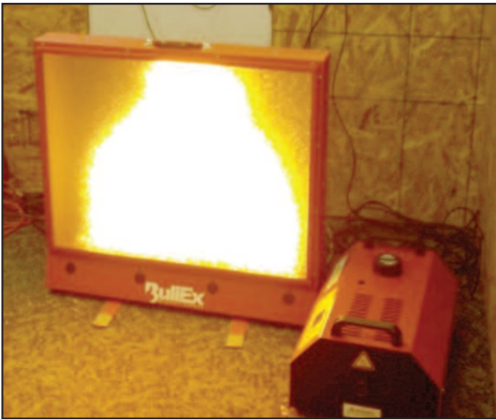
Figure 4: Fire display and smoke generator
