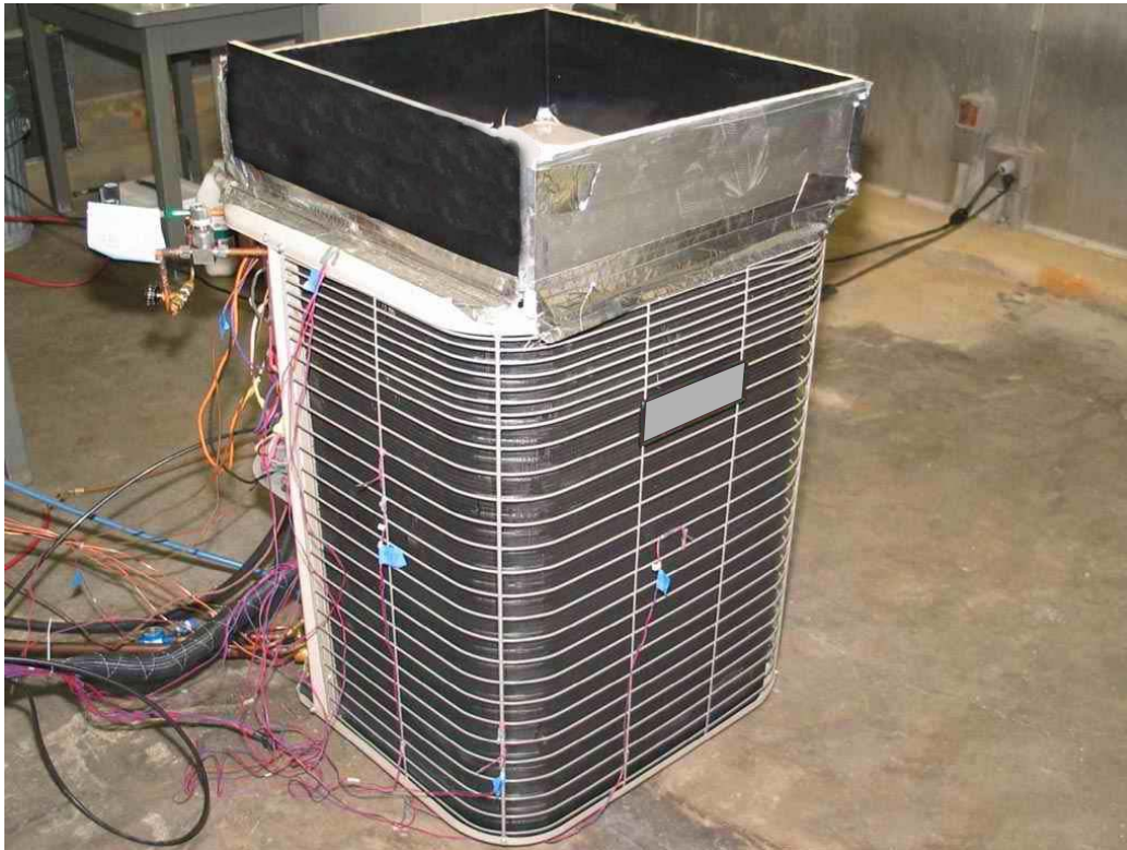
Figure 3.1. Side view of the outdoor section with the flow guide
