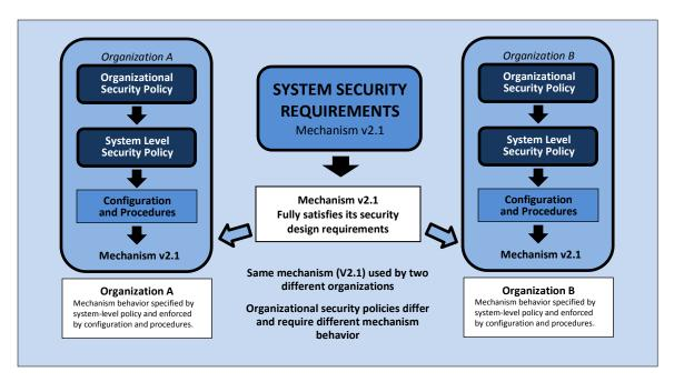
FIGURE G-8: RELATIONSHIP BETWEEN MECHANISMS AND SECURITY POLICY ENFORCEMENT
