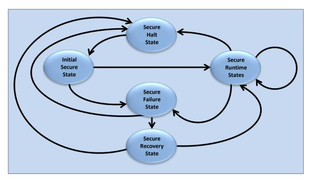
FIGURE G-7: IDEALIZED SECURE SYSTEM STATE TRANSITIONS
