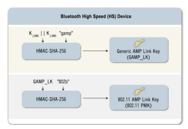
Figure 3-4. AMP Link Key Derivation
