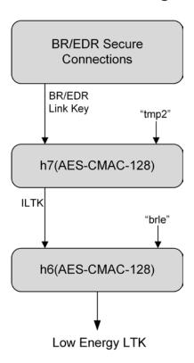
Figure 3-11. Low Energy Long Term Key Derivation from Bluetooth Link Key
