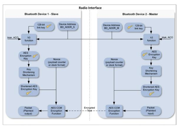
Figure 3-8. Bluetooth AES-CCM Encryption Procedure
