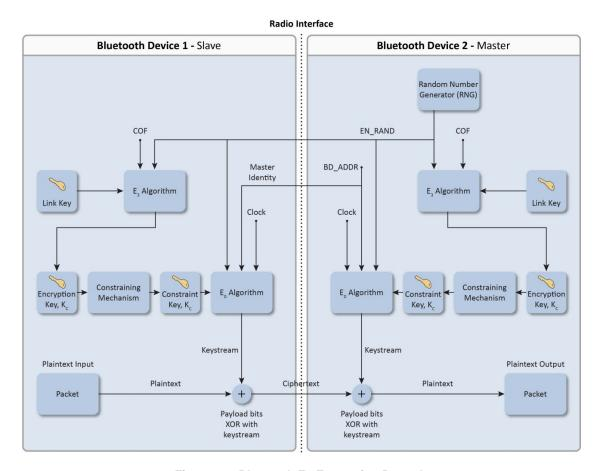
Figure 3-7. Bluetooth E0 Encryption Procedure
