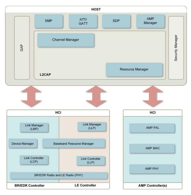
Figure 2-1. Bluetooth 4.x Device Architecture
