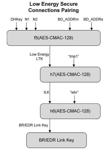
Figure 3-12. Bluetooth Link Key Derivation from Low Energy Long Term Key
