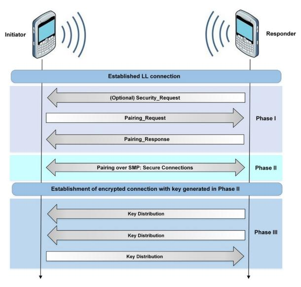
Figure 3-10. Bluetooth Low Energy Secure Connections Pairing
