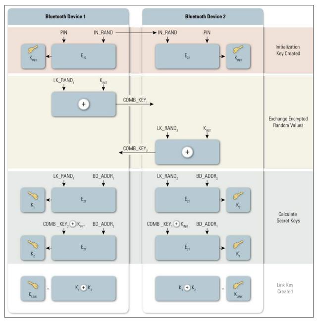
Figure 3-2. Link Key Generation from PIN
