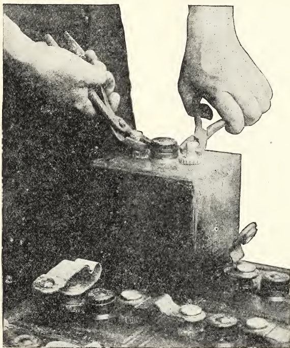
FIG. 37.—Removal of cell from the battery. If the jar sticks, a hot putty knife may be inserted around the edges
