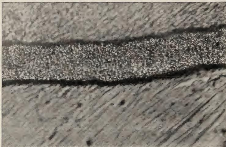
FIG. 10.—Cross section of electrolytic zinc coating, deeply etched with 10 per cent sodium hydroxide. Magnification, 500 diameters
