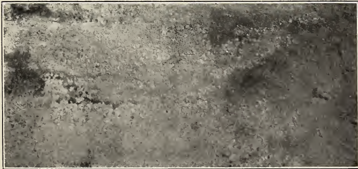
FIG. 3.— Sn-4 solder; 7 days in tap water. \times 1
