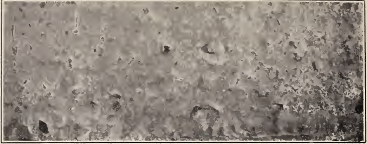
FIG. 4.—Zn-I solder; 7 days in tap water. \times 1
