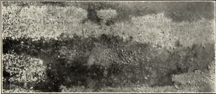
FIG. 2.— Sn-2 solder; 7 days in tap water. \times 1
