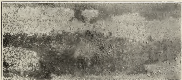
FIG. 2.— Sn-2 solder; 7 days in tap water \times 1
