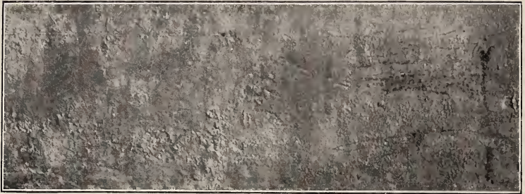
FIG. 5.—Sterling solder; 7 days in tap water. \times 1
