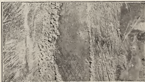
FIG. 7.—Sterling solder joint; photographed wet, showing Al(OH)_3 deposit lines. \times 1
