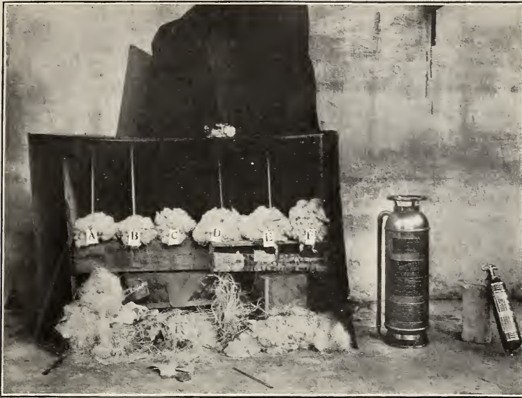
FIG. 21.— Illustrating spontaneous combustion on oily rags and waste Upper sample charred and beginning to smoke
