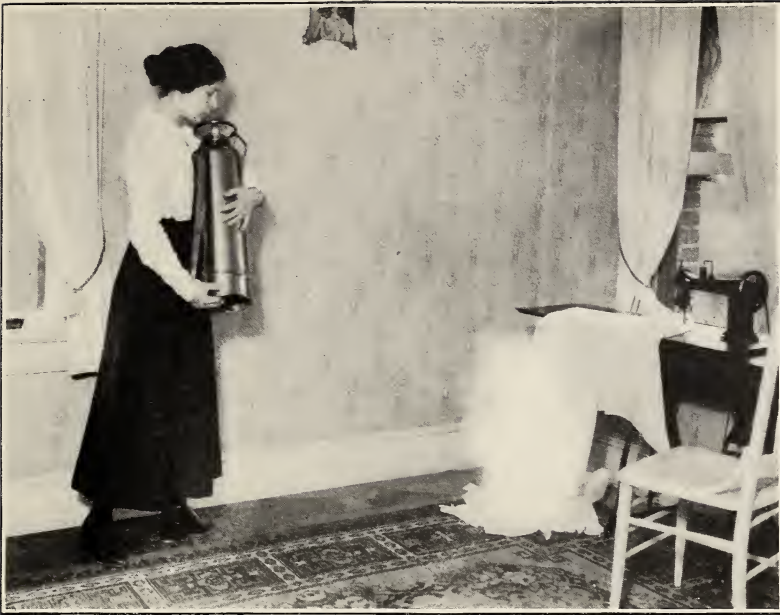
FIG. 24.—Soda-acid fire extinguisher, held upright until fire is reached
