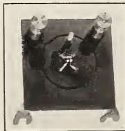
FIG. 111.—Mounted thermocouple with protecting cap removed
