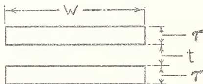
FIG. 212.—Cross section of strip conductors forming a return circuit with narrow surfaces in the same plane
