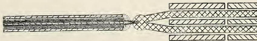
FIGURE 3. Arrangement to assure good thermal contact between the junction of a base-metal thermocouple and that of a protected platinum versus platinum-rhodium thermocouple.
