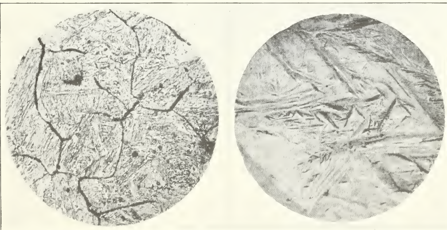
5. C=0.12; Ni=25.0. Quenched from 800° C.; the outlines of the polyhedral austenite crystals show in the matrix of martensite.
