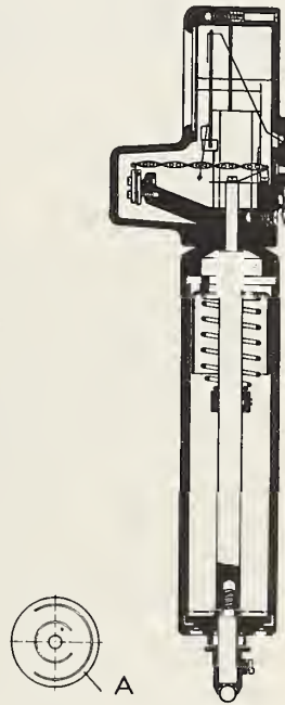
FIGURE 34. Lever magnification of movement.
