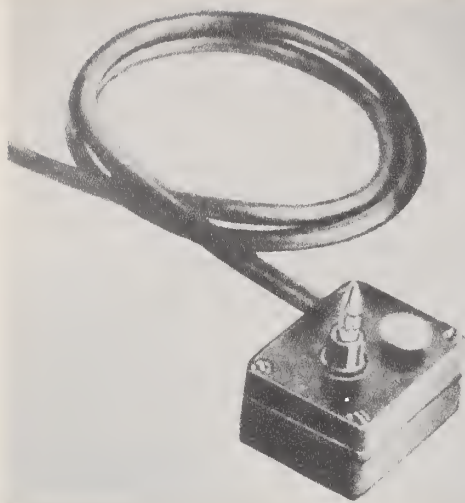
FIGURE 66. Transmitter for electric micrometer.
