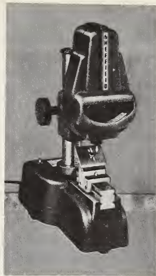
FIGURE 39. "Visual gage," using both mechanical and optical magnification.
