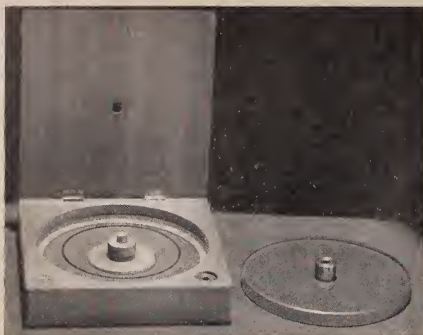
FIGURE 4. Storage box and clamping plug for master circle.
