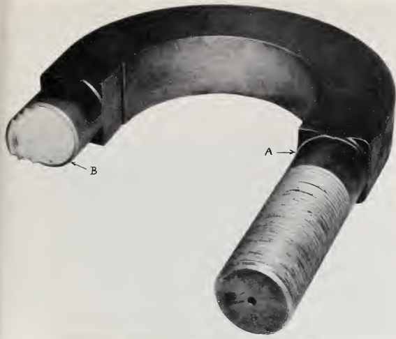
FIGURE 13.1. Fractured yoke with the initial fracture, A fitted together.
