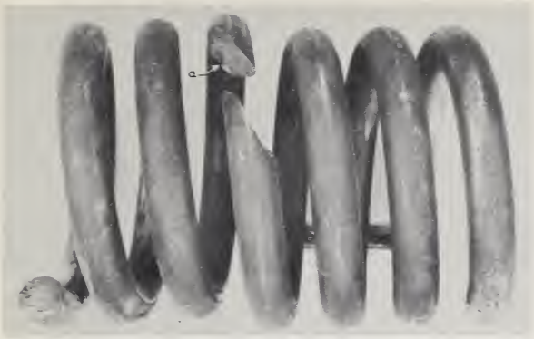
FIGURE 25.1. Fractured helical spring showing the origin of the diagonal fracture on the inside of the coil at arrow "a". \times \frac{1}{2} .
