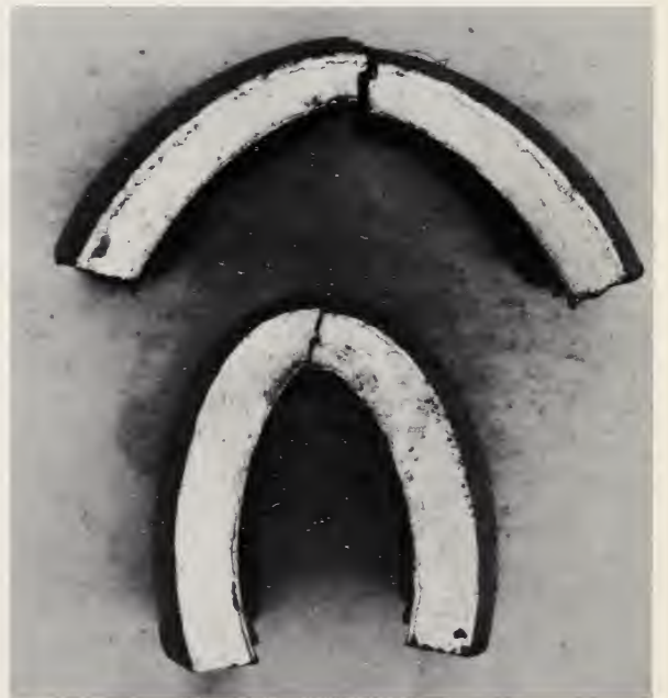
FIGURE 11.3. Bend tests on sections cut from the eye of unused bearings, showing the difference in ductility in different directions.
