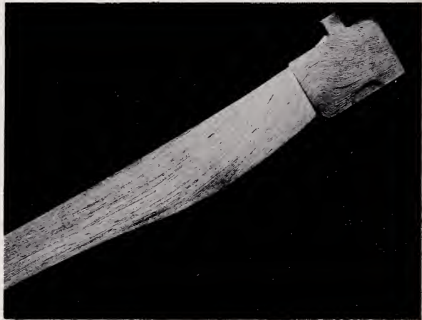
FIGURE 22.4. Longitudinal section of the blade intersecting the fatigue crack.
