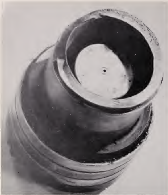
FIGURE 22.1. Hub end of the fractured blade. \times \frac{1}{4} .
