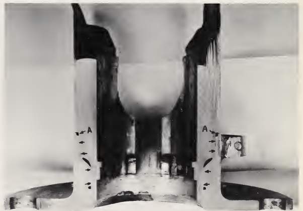
FIGURE 21.2. Cross section of the hub showing the method of assembly.
