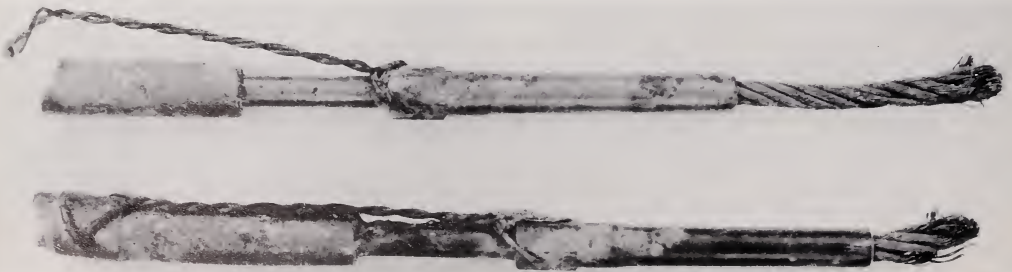
FIGURE 6.1. Parts of two broken turnbuckles removed from a crashed airplane. \times 1 .
