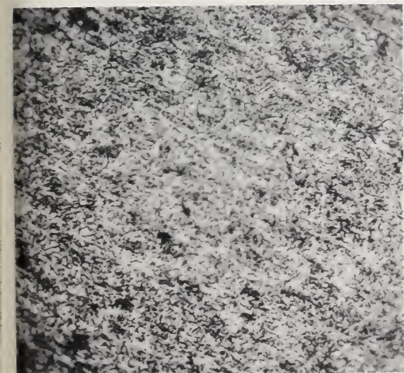
FIGURE 7.2. Microstructure of a longitudinal section of a wire near the fracture indicates that this portion of the cable had been heated sufficiently to spheroidize the carbides and reduce the strength of the cable.
