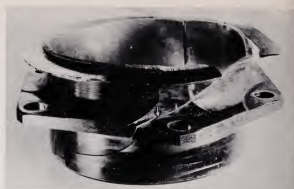
FIGURE 19.1. Lower part of the failed cylinder, showing the fatigue fracture which originated at the cut-out for the hold-down nut, (arrow) and progressed first diagonally, then circumferentially around the cylinder. \times \frac{1}{2} .
