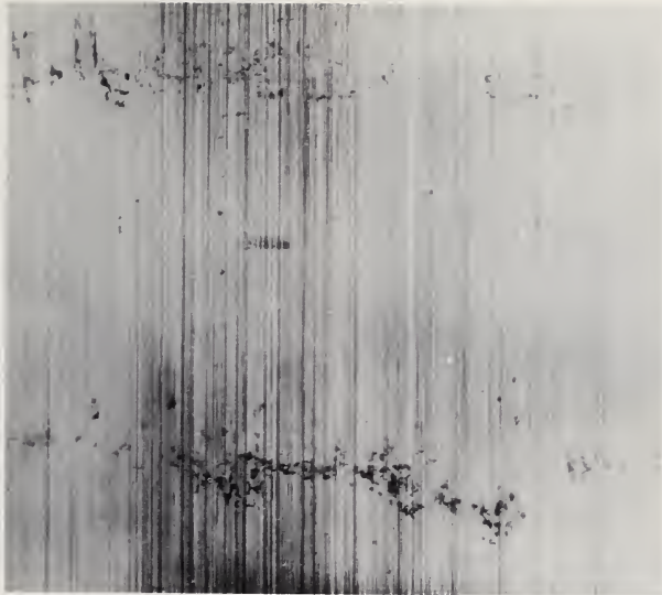
FIGURE 31.4. Corrosion on the surface of the plunger remote from the fatigue crack.
