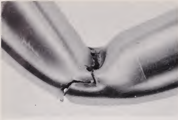
FIGURE 2.1. Fractured piston parts fitted together in approximately the position they had occupied at the time of final fracture.
