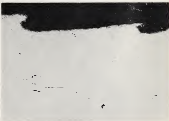
FIGURE 23.4. Longitudinal section through the defect shown in figure 23.3.
