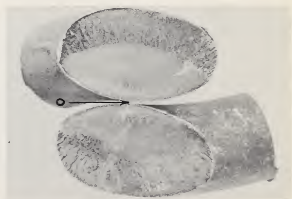
FIGURE 26.2. Surfaces of the fracture; the fatigue crack progressed from the origin at arrow O across nearly half of the section before overload fracture occurred. \times 2 .
