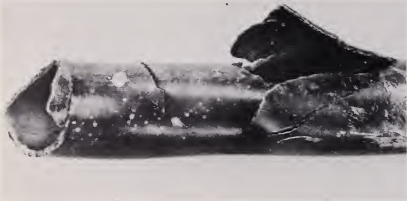
FIGURE 5.1. Failed aluminum-alloy fuel line. \times 1 .
