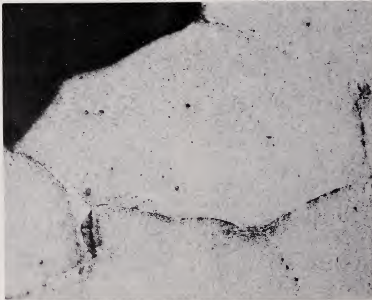
FIGURE 8.3. Microstructure of steel adjacent to the fracture.
