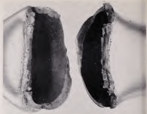
FIGURE 2.2. Fractured surfaces of the tube viewed from the compression side of the bend.
