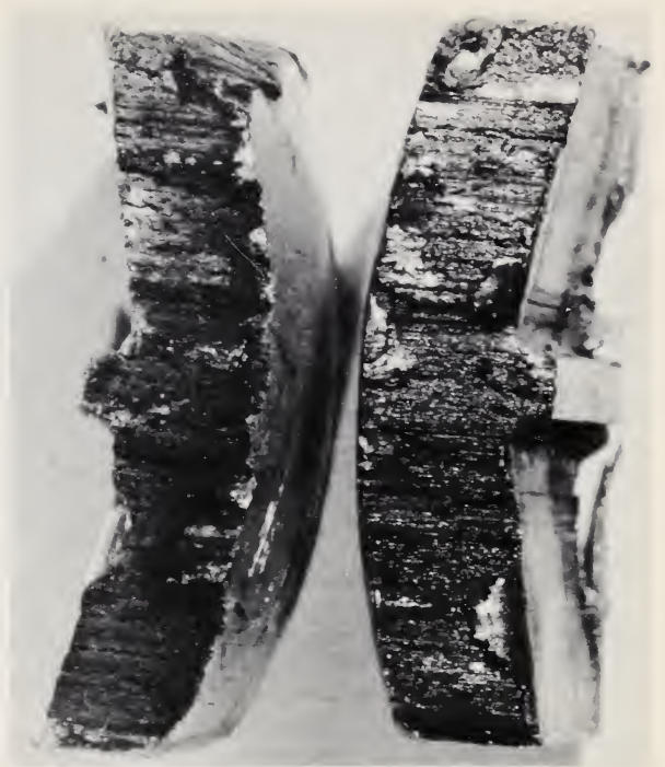
FIGURE 11.2. Surfaces of the fracture; note the "woody" appearance caused by the large number of inclusions in the steel. \times 5 .
