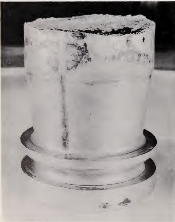
FIGURE 16.2. Surface of the blade near the origin of the fatigue crack.
