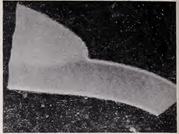
FIGURE 29.2. Transverse section of the tube and weld inboard of the fracture.
