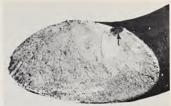
FIGURE 25.2. Fracture surface on one part of the spring. The small dark area (arrow) is the tension fatigue crack which originated at the longitudinal (shear) crack. \times 3 .
