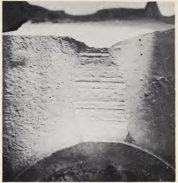
FIGURE 28.2. Bottom surface of the axle adjacent to the fracture, showing the transverse grooves apparently due to shearing off the forging flash.
