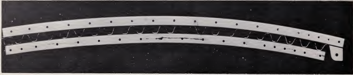
FIGURE 35.1. Cracks in the lower angle as revealed by a dye penetrant inspection method.
