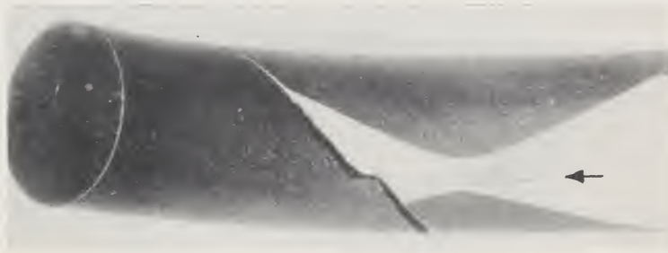
FIGURE 25.3. The two parts of the fracture fitted together. The piece on the right has been ground to show the extent of the longitudinal crack (arrow) away from the fracture. \times 2 .
