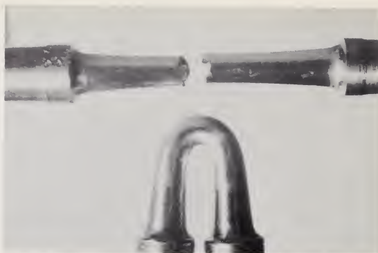
FIGURE 4. Effect of repeated stress on ductility.
