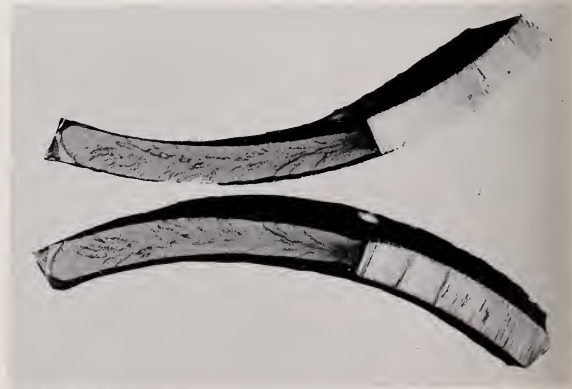
FIGURE 3. Fractured surfaces of specimen shown in figure 2.
