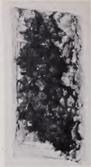
FIGURE 8.2. Surface of the brittle fracture, showing the extremely coarse grains revealed by the fracture. \times 5 .
