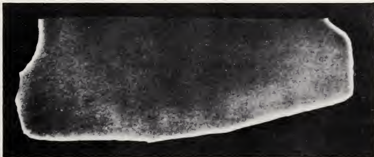
FIGURE 28.3. Section of the lower part of the axle a short distance from the fracture, showing the extensive decarburization of the surface.
