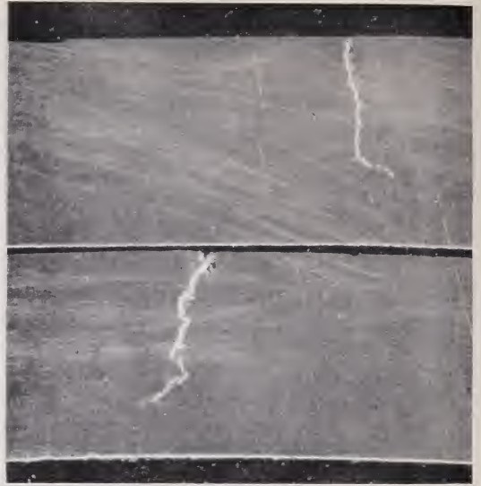
FIGURE 32.3. Cross sections of the tube wall, showing the depth of penetration of the cracks. \times 7 .
