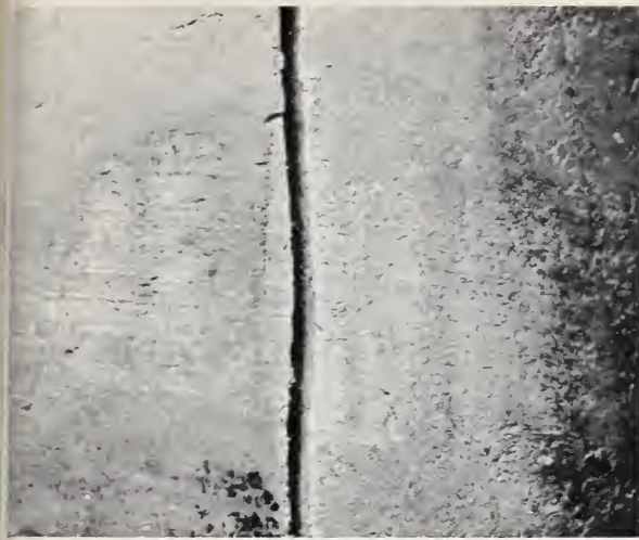
FIGURE 10.3. Surface of the cylinder near the origin of the fracture, showing the abrasions apparently caused by a clamping tool. \times 3 .
