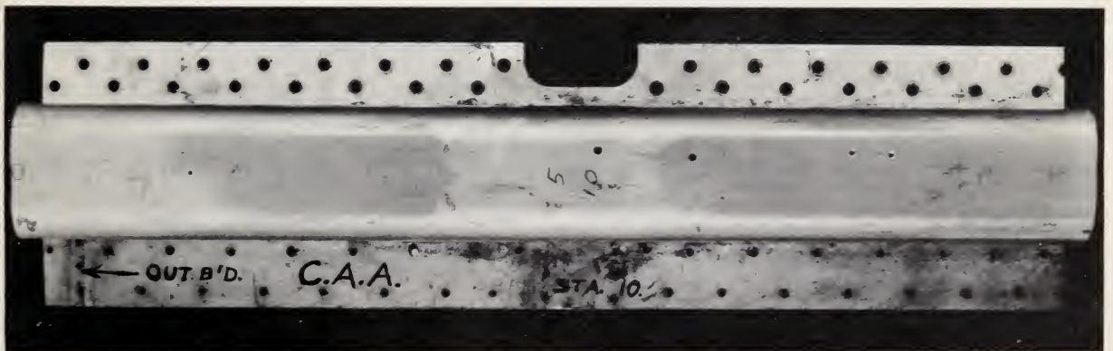
FIGURE 32.1. One of the pieces of cracked spar cap removed from a plane which had been in transoceanic service.
