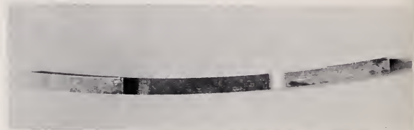
FIGURE 32.5. Specimen that curved when cut from the tube wall as a result of the high internal stress in the part.
