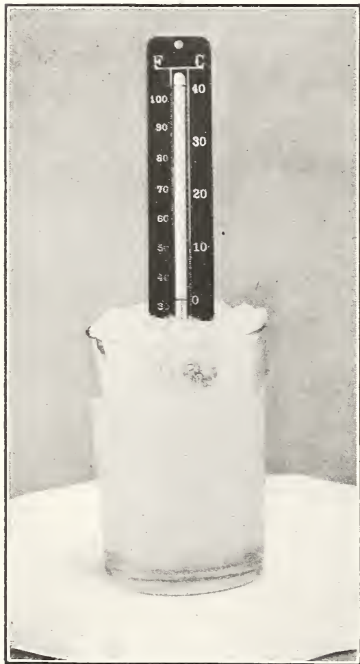
FIG. 12.—Method of testing a thermometer at the freezing point
