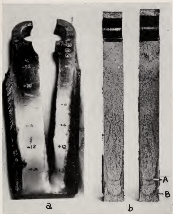
FIGURE 1.15. Test for resistance of steel plate to the spread of a crack.
