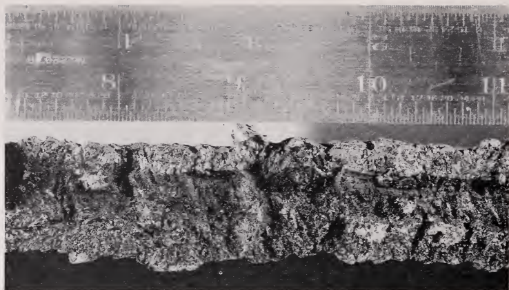
FIGURE 9.3. Fractured weld showing paint penetration in previous crack.
