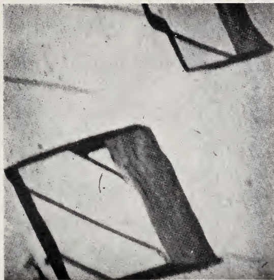
FIGURE 1.9. Slip zones in aluminum at -180^{\circ}\text{C} , \times 10,000 . (A. F. Brown)
