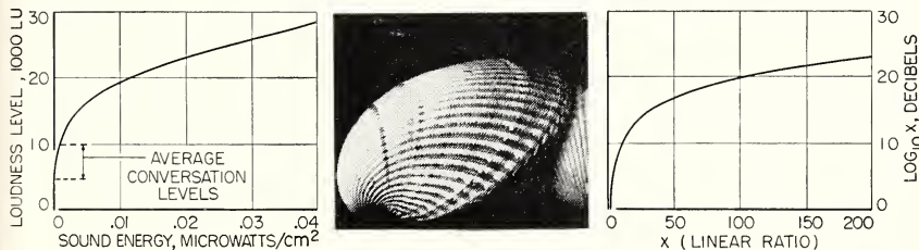
FIGURE 1. As the curve at the left shows, if the energy of a sound is increased, the sensation of loudness perceived by a listener does not increase as rapidly as the increase in energy.
