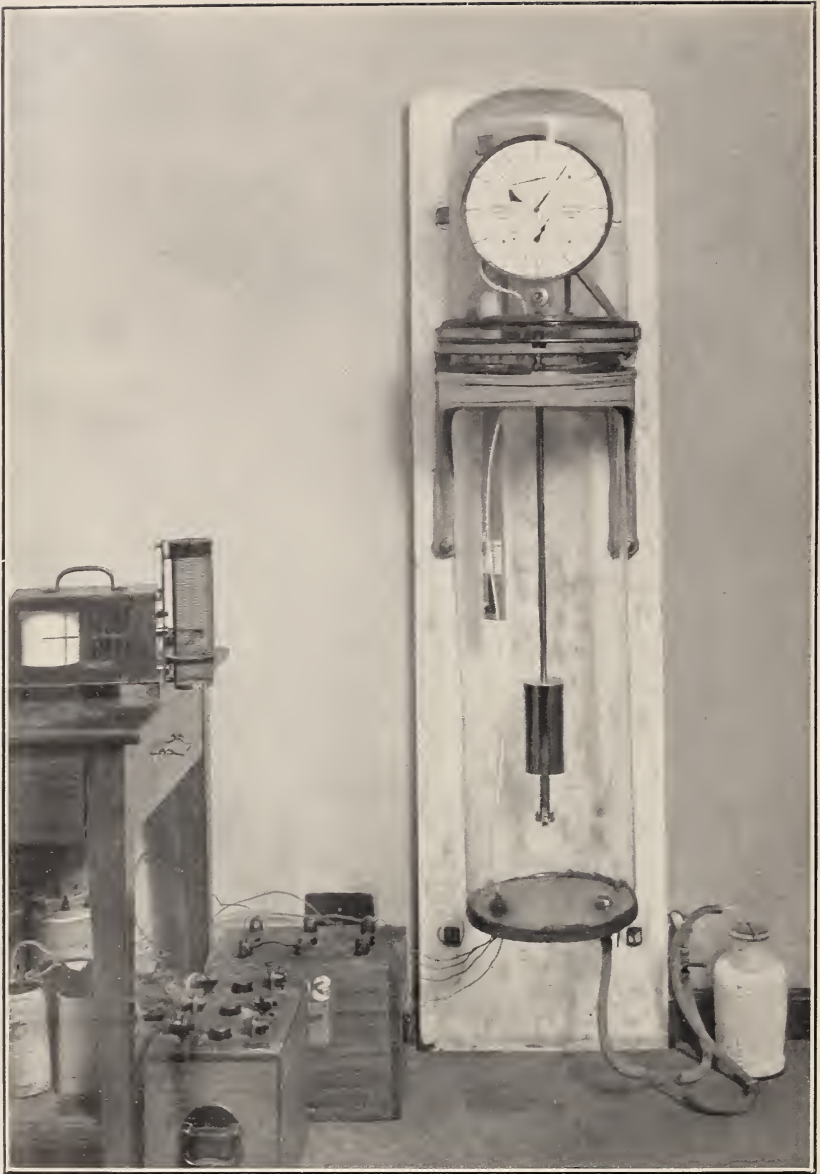
FIG. 1.—Precision mean time clock (Riefler type) used as a standard in the testing of timepieces at the Bureau of Standards
