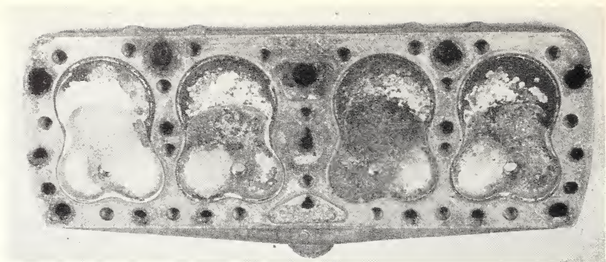
FIGURE 7. Aluminum cylinder head after 734-hour operation on magnesium-chloride antifreeze.
