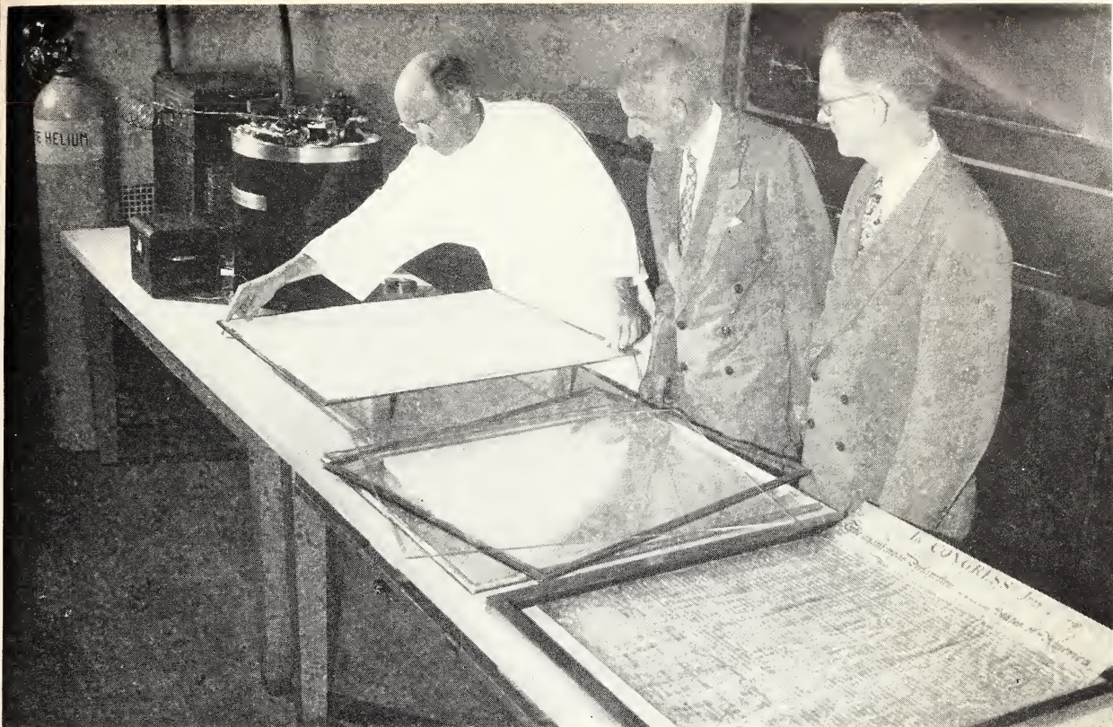
Figure 2.—In the first step of the test sealing of the Declaration of Independence facsimile, backing paper of pure cellulose, made at the National Bureau of Standards, is centered on the bottom panel of tempered glass. This paper serves as a protective cushion for the document and as a reservoir of moisture to prevent excessive changes in relative humidity inside the enclosure. Left to right: Dr. Roy W. Wampler, assistant director of Research, Libbey-Owens-Ford; Mr. Alvin W. Kremer, keeper of the collections, Library of Congress; Dr. G. M. Kline, Chief of Plastics Section, National Bureau of Standards.
