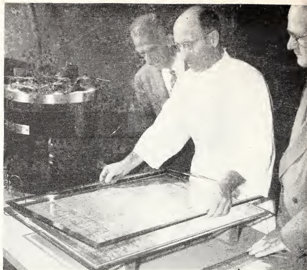
Figure 6.—The bronze bracket around the edge of the cover glass holds the assembly of backing paper, document, and cover glass in position in the enclosure. The bracket also serves to keep the document away from the area heated by soldering during the final sealing operation. Left to right: Mr. A. W. Kremer, Dr. R. W. Wampler, and Dr. G. M. Kline.
