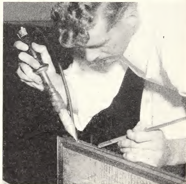
Figure 9.—Tubes are sealed in holes drilled through the lead strip in diagonally opposite corners of the document enclosure to serve as inlet and outlet ports for helium. The ports permit the complete replacement of the air atmosphere around the document with specially humidified helium.
