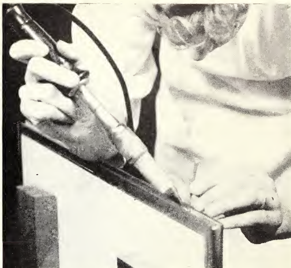
Figure 16.—The constricted tubes, which extend through the lead strip, are removed from the strip and the holes sealed with solder. The facsimile document is now entirely sealed within the test enclosure.
