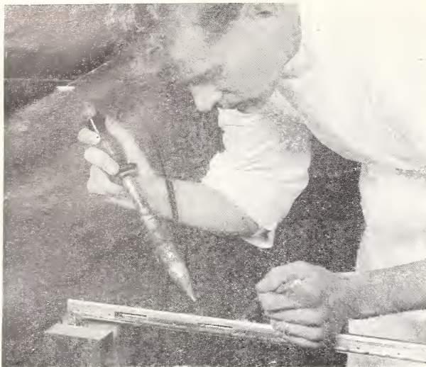
Figure 5.—Before placing the bronze bracket, two leak detector cells are sealed in slots cut in the bracket. These cells detect any change in the composition of the gas within the enclosure. Wires leading to the cells pass through a Kovar tube in which they are fixed by a glass bead. Mr. Louis Gilles of Libbey-Owens-Ford is sealing the Kovar tube in a hole in the lead strip, which is attached to the glass panels of the enclosure.
