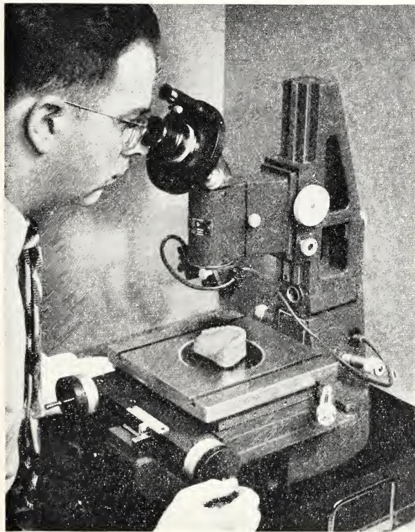
FIGURE 4. Microscope used in making accurate measurements of small changes in the dimensions of artificial dentures.
