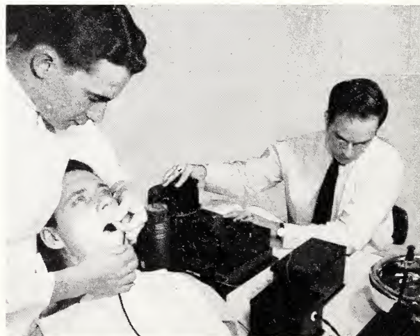
FIGURE 1. Measurement of heat evolved during the hardening of dental restorations.
