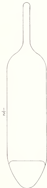
FIGURE 16. Float for determination of density of liquids, one-half size (Warrington).
