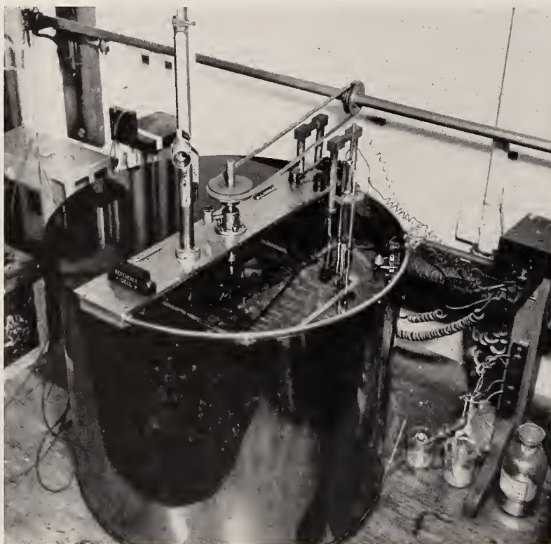
FIGURE 6. Primary group of standard cells in oil bath.
