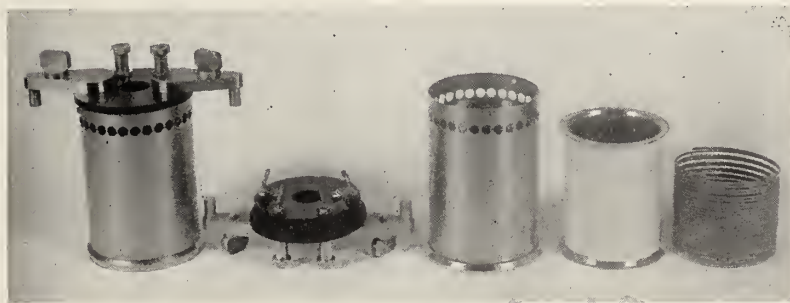
FIGURE 4. Double-walled (Thomas type) standard resistor.
